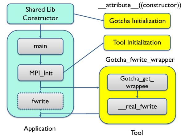
Fig 2. Modified control flow of an end-user application when using a Gotcha enabled tool with it.
