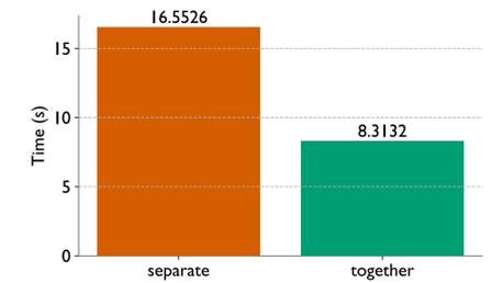
Fig 5. Time spent in getting both Recorder & Darshan profiles when the tools are used separately versus used together in the same run.
